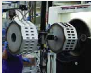
5 Vacuum Metallizing Reflector Machines
