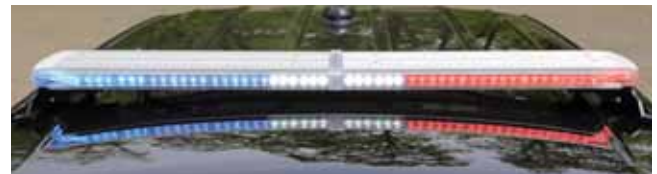
Complete light coverage with no dead spots between modules.
